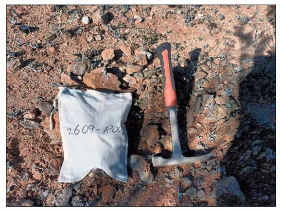
Rock Sample 2609-R001 contained fine disseminated chalcopyrite and very minor pyrite cuboid crystals.
